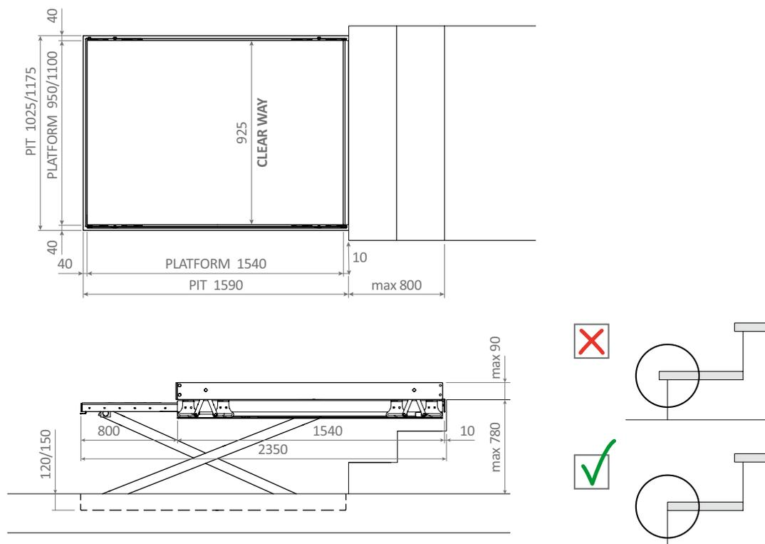
\* version with the column (optional) with altitude difference  $\leq 500$  mm without protective bellows (supplied as standard).
